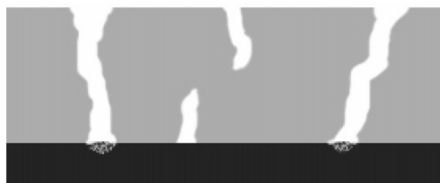
Figure 1. Schematic drawing of a Nafion polymer membrane with hydrophilic channels (white) affixed to a silicon substrate (black). A percentage of the channels traverse the entire membrane, allowing electrochemical etching at the Nafion/silicon interface. This method of selective electrochemical etching initiates porous silicon (speckled gray) at the location of the hydrophilic channels.
